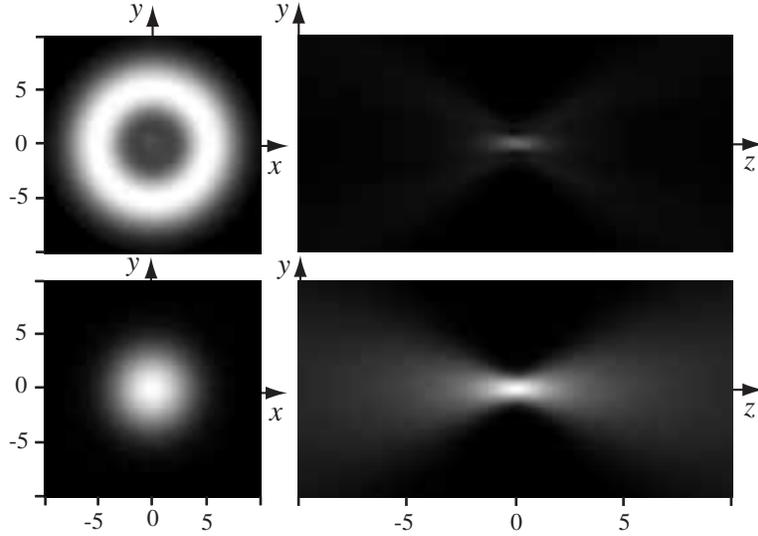
Fig. 4. Intensity distribution of the LCP beam (top) and a reference linearly polarized Gaussian beam (bottom). The distributions in the meridional plane  $x = 0$  (right) and the transverse plane  $z/z_0 = -5$  (left) are shown. The axial position  $z$  is in units of  $z_0$  and the transverse dimensions are in units of  $W_0$ . The offset ratio  $r = \Delta/z_0 = 0.25$ . In each figure, the intensity is normalized such that the maximum value is unity.
