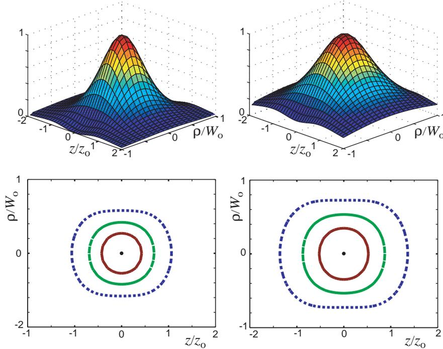
Fig. 6. Intensity distributions (above) and contours of constant intensity (below) for the minority component (left) and the reference Gaussian beam (right). The contours are at fractions of the peak intensity of 2/3 (solid red line), 1/2 (dashed green line), and 1/3 (dotted blue line).
