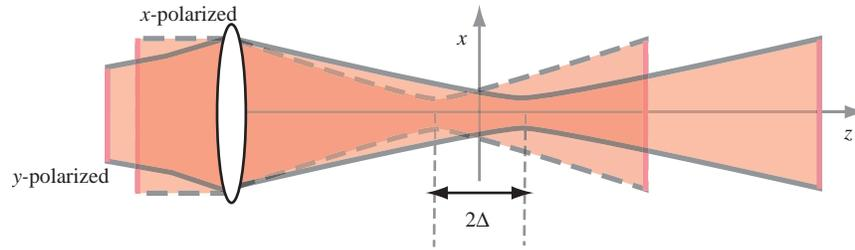
Fig. 5. Proposed scheme for creating polarization-assisted superresolution. Two Gaussian beams of the same width and with a slight difference in curvature are focused by a lens. The  $x$ - and  $y$ -polarized components have a  $90^\circ$  phase shift at the beam axis. The left-circularly polarized component (minority) is highly confined in the focal region.
