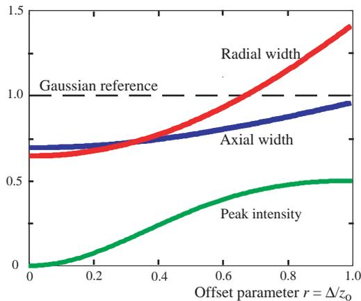
Fig. 3. Dependence of the axial and radial widths (FWHM) and the peak intensity of the LCP (minority) component on the offset parameter  $r = \Delta/z_0$ . All values are normalized to the corresponding values for the constituent Gaussian beam.
