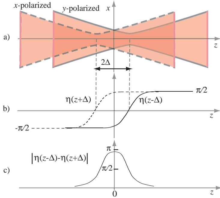
Fig. 1. (a) Superposition of x- and y-polarized coaxial Gaussian beams with centers offset by a distance  $2\Delta$ . (b) The Gouy phase shifts associated with the two beams. (c) Difference of the Gouy phases.
