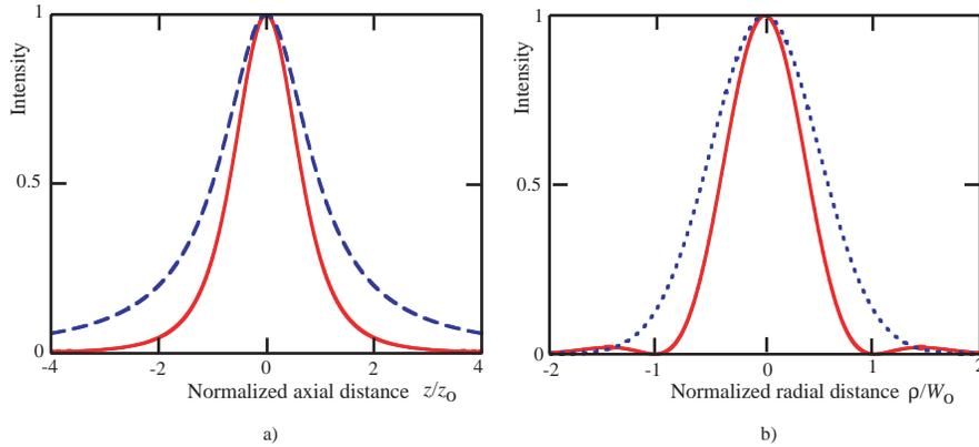
Fig. 2. (a) Axial distributions of the LCP component (solid curve) and the constituent Gaussian linearly polarized beam (dashed). (b) Radial distributions of the LCP component (solid curve) and the constituent Gaussian linearly polarized beam (dashed).
