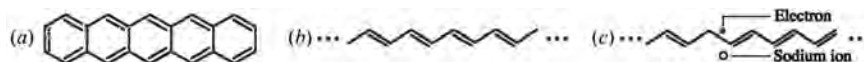
Figure 5.9-1 Organic semiconductors for photonics exist in two main variants: (a) small organic molecules (e.g., pentacene), and (b) conjugated polymer chains (e.g., polyacetylene). (c) Doping polyacetylene with \text{Na}^+ donors yields an n -type material, whereas doping with \text{I}^- acceptors yields a p -type material. In the representation displayed in the figure, each vertex represents a carbon atom, each line represents a bond between two carbon atoms, and each double line represents a double bond. Hydrogen bonds are omitted for clarity.
