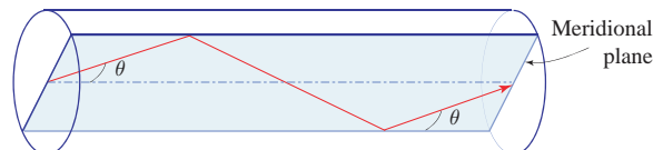
Figure 1.6-4 The trajectory of a meridional ray lies in a plane that passes through the fiber axis. The ray is guided if \theta < \bar{\theta}_c = \cos^{-1}(n_2/n_1) .
