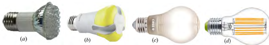
Figure 11.4-1 Evolution of the white LED retrofit lamp from 2004 to 2024. LED lamps, including those shown here, generally contain multiple LEDs. (a) Cool-white DIP LED retrofit spot lamp (ca. 2005). (b) Philips warm-white L-prize LED retrofit lamp (ca. 2011). (c) Contemporary warm-white SMD LED retrofit lamp (ca. 2020). (d) Contemporary neutral-white, ultra-efficient, LED-filament retrofit lamp (ca. 2024).
