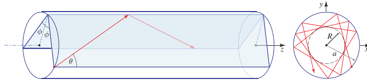
Figure 1.6-5 A skewed ray lies in a plane offset from the fiber axis by a distance R . The ray is identified by the angles \theta and \phi . It follows a helical trajectory confined within a cylindrical shell whose inner and outer radii are R and a , respectively. The projection of the ray on the transverse plane is a regular polygon that is not necessarily closed.
