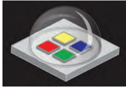
Figure 11.3-2 Sketch of a CMLED, a multicolor color-mixing LED comprising individually addressable red, green, and blue dies, along with a white phosphor-conversion emitter of selectable CCT. The dies are housed within a ceramic surface-mounted device (SMD) capped by a 5-mm-diameter hemispherical lens. CMLEDs such as this can be electrically tuned to emit essentially any color within the gamut of human vision, including metameric white light.
