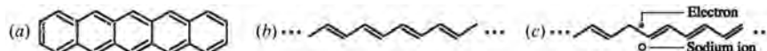
Figure 5.9-1 Organic semiconductors for photonics exist in two main variants: (a) small organic molecules (e.g., pentacene), and (b) conjugated polymer chains (e.g., polyacetylene). (c) Doping polyacetylene with \text{Na}^+ donors yields an n -type material, whereas doping with \text{I}^- acceptors yields a p -type material. In the representation displayed in the figure, each vertex represents a carbon atom, each line represents a bond between two carbon atoms, and each double line represents a double bond. Hydrogen bonds are omitted for clarity. Various types of organic molecules and polymers find use in photonics.
