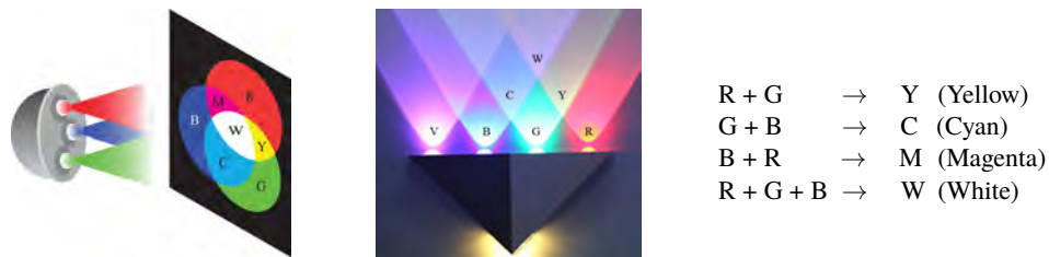
Figure 11.3-1 Additive color mixing. Left: A device that generates light of tunable color can be constructed from LEDs that emit light in the Red (R), Green (G), and Blue (B), as schematically illustrated. Center: Light produced by a wall sconce constructed from LEDs that emit, from left to right, Violet (V), Blue, Green, and Red. (Adapted from Wandlampe by Mattes, 4 July 2018, via Wikimedia Commons.) Right: The color-mixing rules specified in the table delineate the colors exhibited in the images at left and center. The yellow (Y), cyan (C), and white (W) generated by the wall sconce exhibit limited brightness because of reduced luminance, as exemplified in Examples 9.3-1–9.3-3.
