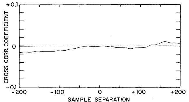
Fig. 2. Cross-correlation coefficient between the in-phase and quadrature components of computer-simulated Gaussian-Lorentzian radiation as a function of Nyquist sample separation. It can be seen that the absolute value of the coefficient is always considerably less than unity, indicating that the two components are virtually uncorrelated.
