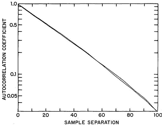
Fig. 1. Autocorrelation coefficients of the in-phase and quadrature components of computer-simulated Gaussian-Lorentzian radiation as a function of Nyquist sample separation. As expected, the two curves are very similar and appear as virtually straight lines on a log-linear plot, corresponding to an exponential falloff.
