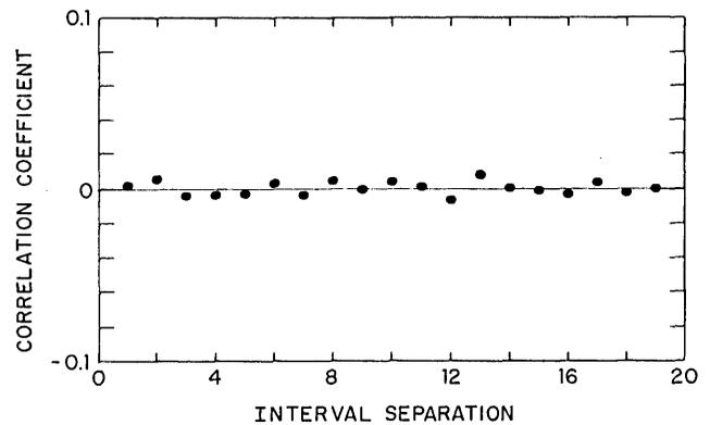
Fig. 4. Statistics of photons from a light-emitting diode (LED). Correlation between interphoton intervals for different interval separations. The first data point corresponds to consecutive intervals, whereas the last data point corresponds to intervals separated by eighteen intervening intervals. Observe that no correlation point exhibits an absolute value larger than 0.01.
