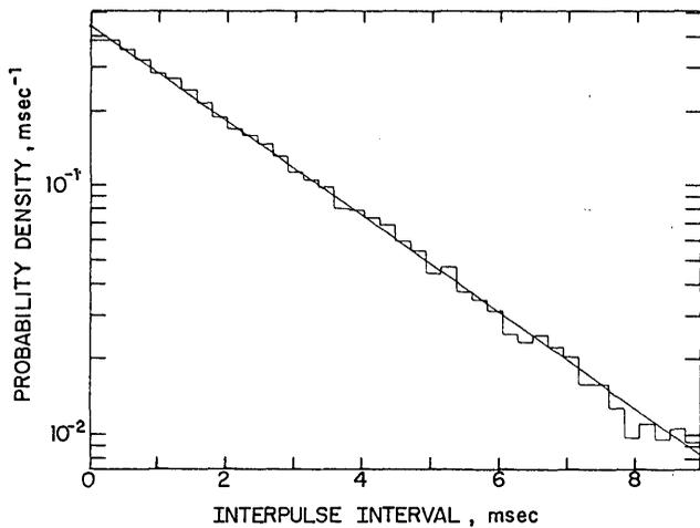
Fig. 3. Statistics of photons from a light-emitting diode (LED). Experimental histogram and theoretical distribution of the time interval between consecutive detected photons. The solid straight line represents the theoretical (exponential) probability density function for a Poisson point process with constant rate. The mean time interval is 2.25 msec.
