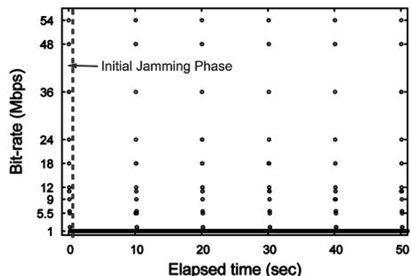
Fig. 4: Performance of SampleRate under bursty periodic jamming with  $a = 44$  and  $T = 934$ .  $Thr = 0.955$  Mb/s.
