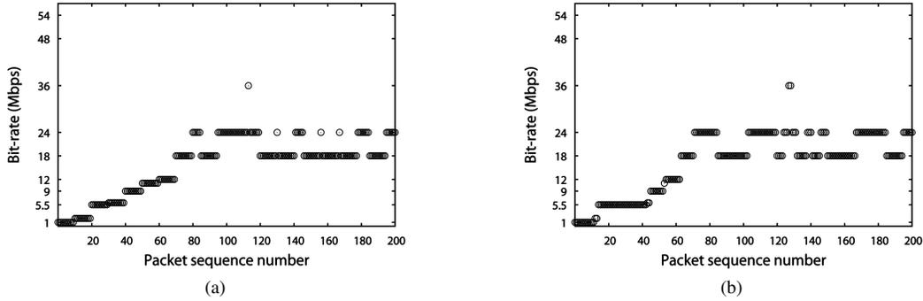
Fig. 5: Performance under lossy channel with no jamming: (a) ARF,  $Thr = 21.77$  Mb/s, (b) RARF,  $Thr = 23.22$  Mb/s. ARF and RARF perform similarly under lossy channel conditions in the absence of a jammer.
