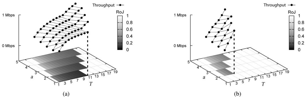
Fig. 3: Throughput of (a) ARF and (b) RARF under periodic jamming with parameters  $a$  and  $T$ .  $RoJ$  is depicted as a contour plot at the bottom of each graph. Low  $RoJ$  values are plotted in dark colors to indicate the severity of the vulnerability. Among the strategies to keep the throughput below 1 Mb/s, the one with the lowest  $RoJ$  is indicated.
