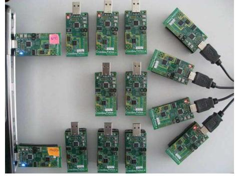
Fig. 5. Tmote Sky sensors testbed with 14 motes.
