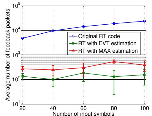
Fig. 9. Expected number of feedback packets while varying the number of input symbols.  $M = 100$  input packets, packet loss rates are distributed uniformly at random from 10% to 20%, varying the number of receivers. 95% confidence interval. Averaged over 100 iterations.
