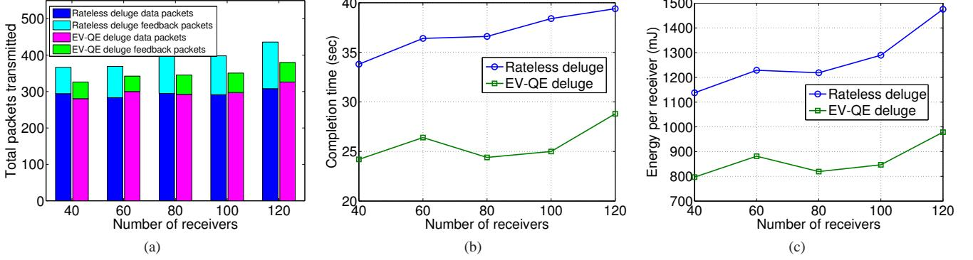
Fig. 7. Rateless Deluge vs. EV-QE Deluge, TOSSIM simulation: 9 pages,  $M = 20$ , heterogeneous packet loss, varying the number of receivers  $N$ . (a) Total packets transmitted: forward and feedback channels, (b) Completion time, (c) Average energy consumption per receiver.
