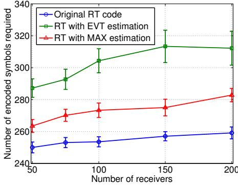
Fig. 10. Original RT vs. modified RT, expected completion time.  $M = 100$  input packets, packet loss rates are distributed uniformly at random from 10% to 20%, varying the number of receivers. 95% confidence interval. Averaged over 100 iterations.
