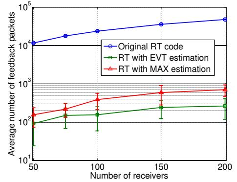
Fig. 11. Expected number of feedback packets while varying the number of receivers.  $M = 100$  input packets, packet loss rates are distributed uniformly at random from 10% to 20%, varying the number of receivers. 95% confidence interval. Averaged over 100 iterations.
