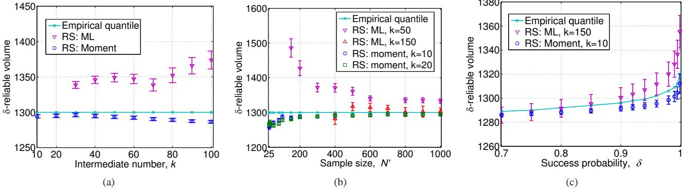
Fig. 3. Performance of extreme value FEC redundancy estimators for different parameters, with 95% confidence interval. (a)  $N' = 1000$ ,  $\delta = 95\%$ , varying  $k$ , (b)  $\delta = 95\%$ , varying  $N'$ , (c)  $N' = 1000$ , varying  $\delta$ .
