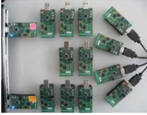
Fig. 4. Tmote Sky sensors testbed with 14 motes.
