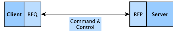
Fig. 13. The command and control message system (a subset of the data flow laid out in Figure 5).
