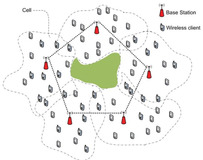
Fig. 1. Illustration of a wireless cellular network. Wireless clients are connected to base stations (clusterheads), which are interconnected via reliable wireline/wireless links themselves. The dotted irregular shapes contour radio signal range of each clusterhead. It is assumed that one or more of the clusterhead is connected to greater networks (not shown in the figure).
