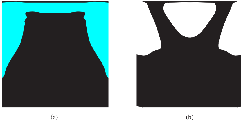
Fig. 11. Optimal topology for \bar{F}_{1112} : (a) PZT/polymer; (b) PZT/void.
