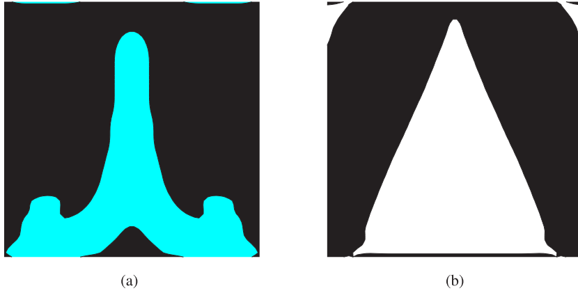
Fig. 10. Optimal topology for \bar{F}_{2221} : (a) PZT/polymer; (b) PZT/void.
