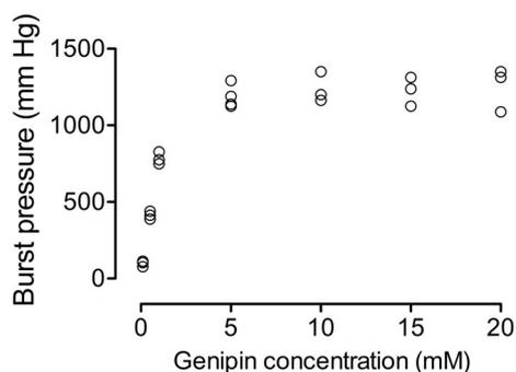
**FIGURE 4** Plot of burst pressure of collagen tubes as a function of crosslinker concentration
