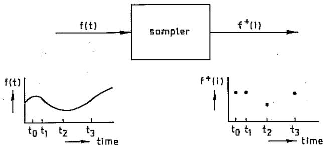
Fig. 6.1. Continuous-to-discrete-time conversion.
