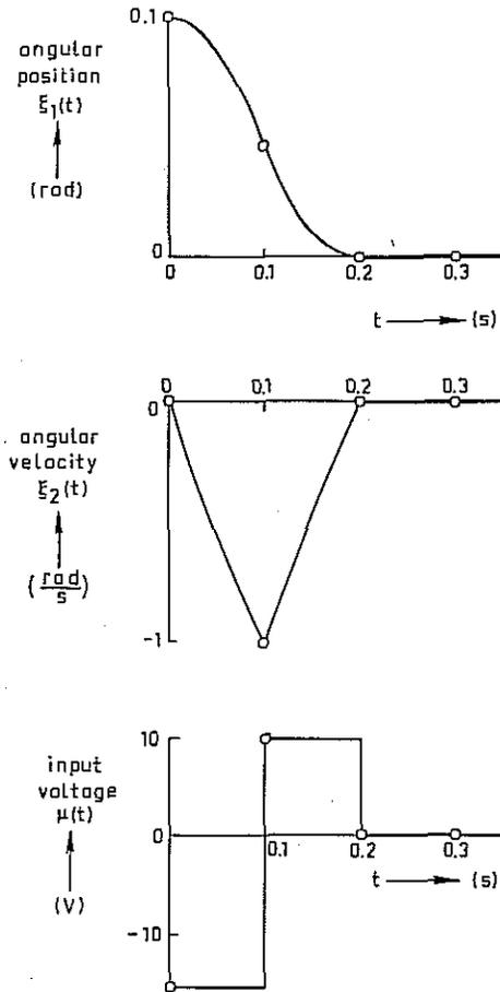
Fig. 6.12. State deadbeat response of the digital position control system.
