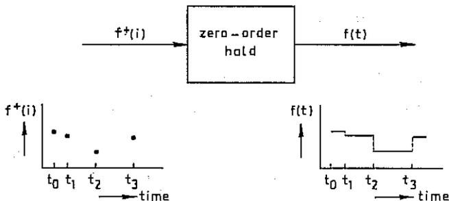
Fig. 6.2. Discrete-to-continuous-time conversion.
