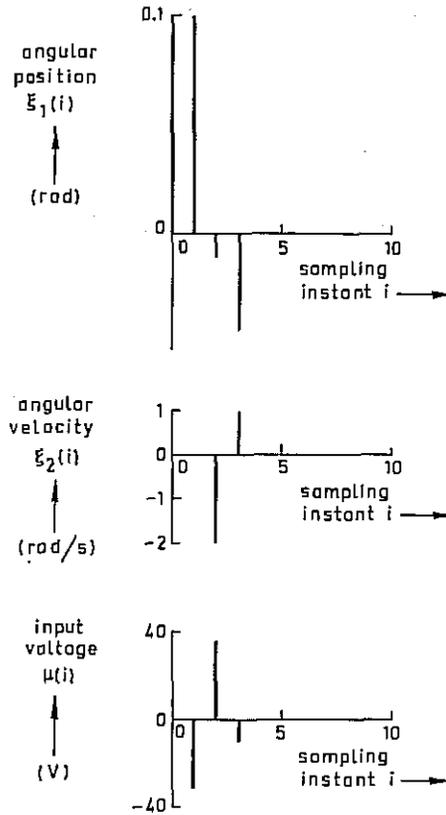
Fig. 6.22. Response of the output feedback state deadbeat position control system from the initial state  $\text{col}[x(0), \hat{x}(0)] = \text{col}(0.1, 0, 0, 0)$ . The responses are shown at the sampling instants only and not at intermediate times.
