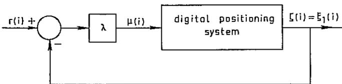
Fig. 6.7. A digital positioning system with proportional feedback.
