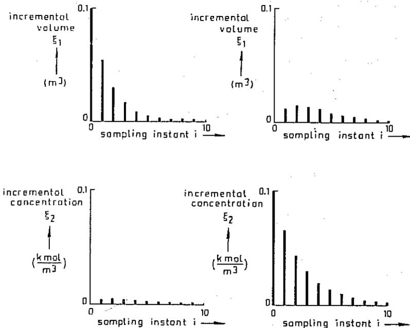
Fig. 6.14. Closed-loop responses of the regulated stirred tank, discrete-time version. Left column: Responses of volume and concentration to the initial conditions  $\xi_1(0) = 0.1 \text{ m}^3$  and  $\xi_2(0) = 0 \text{ kmol/m}^3$ . Right column: Responses of volume and concentration to the initial conditions  $\xi_1(0) = 0 \text{ m}^3$  and  $\xi_2(0) = 0.1 \text{ kmol/m}^3$ .
