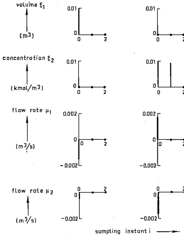
**Fig. 6.18.** Deadbeat response of the stirred tank with time delay. Left column: Responses of volume, concentration, feed no. 1, and feed no. 2 to the initial condition  $\xi_1(0) = 0.01 \text{ m}^3$ , while all other components of the initial state are zero. Right column: Responses of volume, concentration, feed no. 1, and feed no. 2 to the initial condition  $\xi_2(0) = 0.01 \text{ kmol/m}^3$ , while all other components of the initial state are zero.
