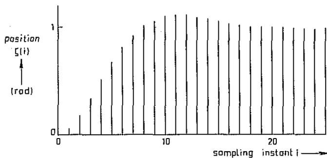
Fig. 6.11. The response of the digital position control system to a step in the reference variable of 1 rad.
