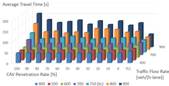
Fig. 8: Average travel time with respect to different traffic flow rates and CAV penetration rates.
