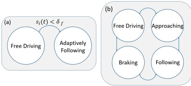
Fig. 3: (a) Modeling approach for CAVs; (b) The Wiedemann model for non-CAVs.
