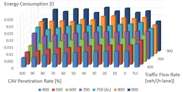
Fig. 7: Average energy consumption with respect to different traffic flow rates and CAV penetration rates.
