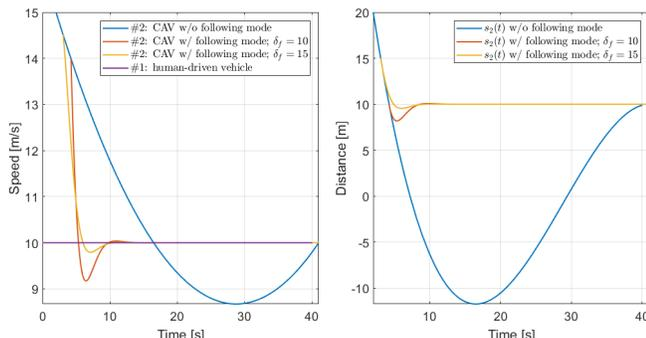
Fig. 4: Speed  $v_i(t)$  and inter-vehicle distance  $s_2(t)$  trajectories w/ and w/o the optimal control for adaptively following.
