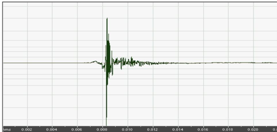
**Figure 5.5:** Measured impulse response of the ESS measurement system. Time-scale: 2 ms per division; amplitude-scale: 3 dB per division. Reproduced, with kind permission from IEEE, from D. Frey, V. Coelho, and R.M. Rangayyan, “Filtering and removal of the effects of the transducers on the acoustical impulse response of concert halls,” *IEEE Canadian Conference on Electrical and Computer Engineering (CCECE)*, St. John’s, Newfoundland and Labrador, Canada, 3–6 May, 2009, pp. 368–371. © IEEE.
