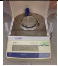
Zero the balance and put the calibrated weight on the weighing pane. Please wear gloves when handle the weight.
