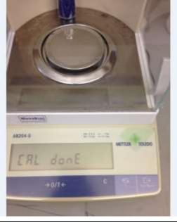
6. When calibration is done correctly, the screen will show " CAL done".
