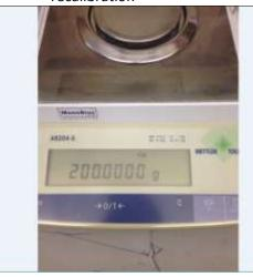
4. When "200.0000 g" bilking, put the calibrated weigh on the weighing pane, close the door
