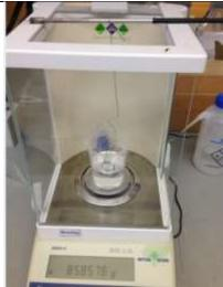
5. Dip empty mesh basket in water, not touching any walls, do not overload balance! Use less than 100mL water
