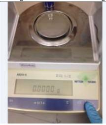
3. Press calibration key when nothing is on the balance and you will see "cal" blinking
