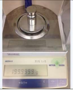
7. Check the reading with calibrated weight.
