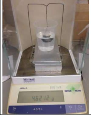
Move plastic container with sufficient water to dip specimen in water, do not spill water. Make sure speciem is immersed. Remove air bubbles but do not remove any water. Recode w2 = 4.6212 g
