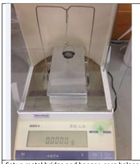
Setup metal bridge and hanger, zero balance
