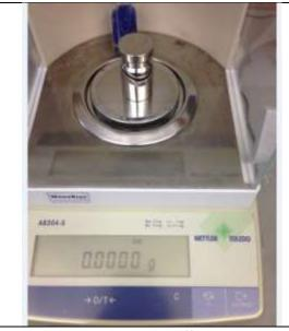
5. When the binking goes off automatically and "0.0000 g" starts blinking, take the weight away.
