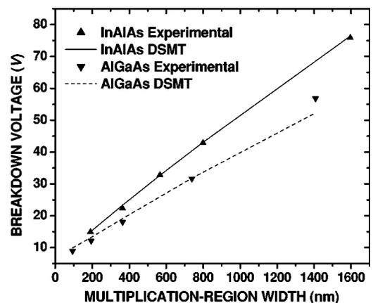
FIG. 2. Experimentally measured breakdown voltage  $V_B$  versus multiplication-region width  $w$  for In<sub>0.52</sub>Al<sub>0.48</sub>As (triangles) and Al<sub>0.2</sub>Ga<sub>0.8</sub>As devices (inverted triangles). Predictions based on the DSMT are shown as solid and dashed curves for InAlAs and AlGaAs, respectively.
