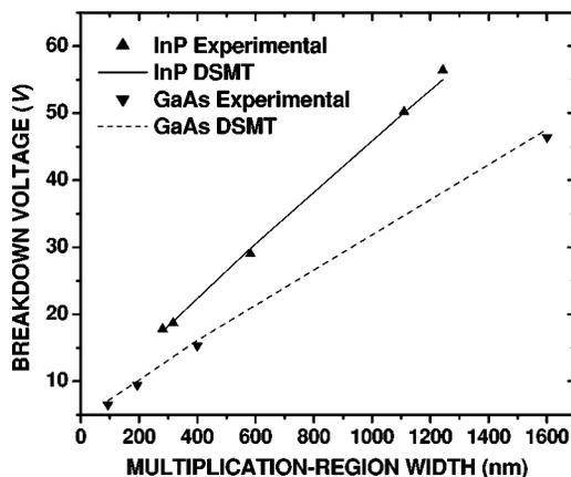
FIG. 1. Experimentally measured breakdown voltage  $V_B$  versus multiplication-region width  $w$  for InP (triangles) and GaAs devices (inverted triangles). Predictions based on the DSMT are shown as solid and dashed curves for InP and GaAs, respectively.
