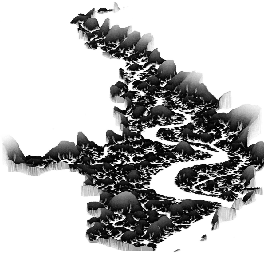
Figure 2. The vertically exaggerated water surface topography derived from solving equation (3) by assuming K = 1 for the Petaluma Marsh study area (depicted in Figure 3 of Fagherazzi, et al. [this issue]). The choice of the constant K is immaterial for the delineation of drainage directions because of the linearity of the mathematical solution. Notice the membrane-like features of the potential field that uniquely define drainage directions.
