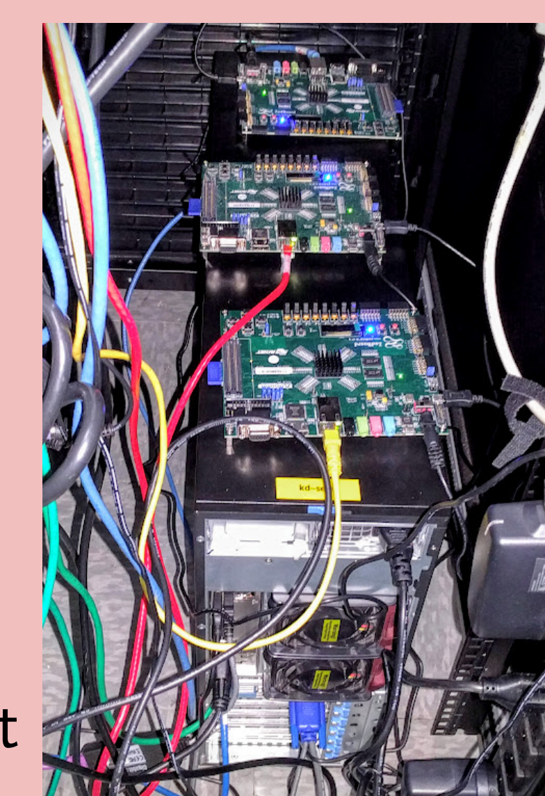
Figure 4: Three Rocket + X-FILES/DANA FPGAs attached to a server
