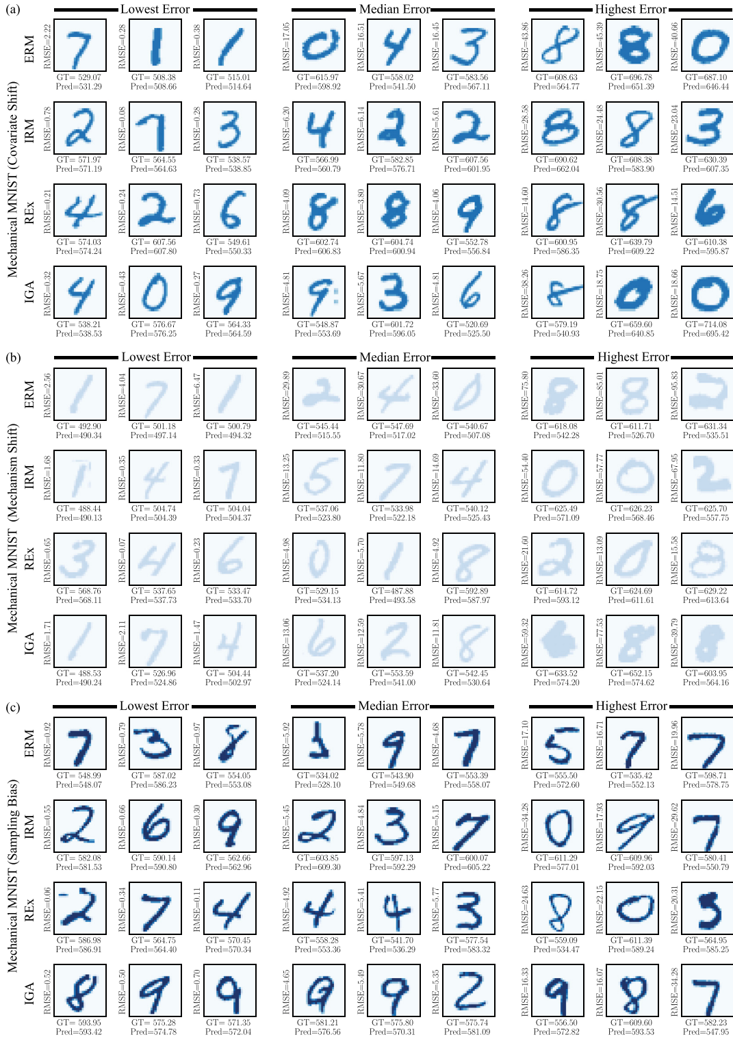
Fig. 18. The sampled cases of three groups: lowest error (bottom 10% RMSE), median error (45% – 55% RMSE) and highest error (top 10% RMSE) from the Mechanical MNIST collection and the corresponding ground truth and prediction of the change in strain energy. For each OOD dataset (a) Covariate Shift (b) Mechanism Shift and (c) Sampling Bias, the error (RMSE) is calculated and sorted based on the predicted value given by LeNet model on ERM, IRM, REX, and IGA respectively.
