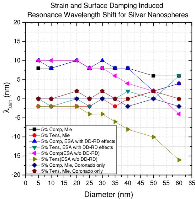
**Figure 1.** Strain-induced shift in the plasmon resonance wavelength for scattering.
