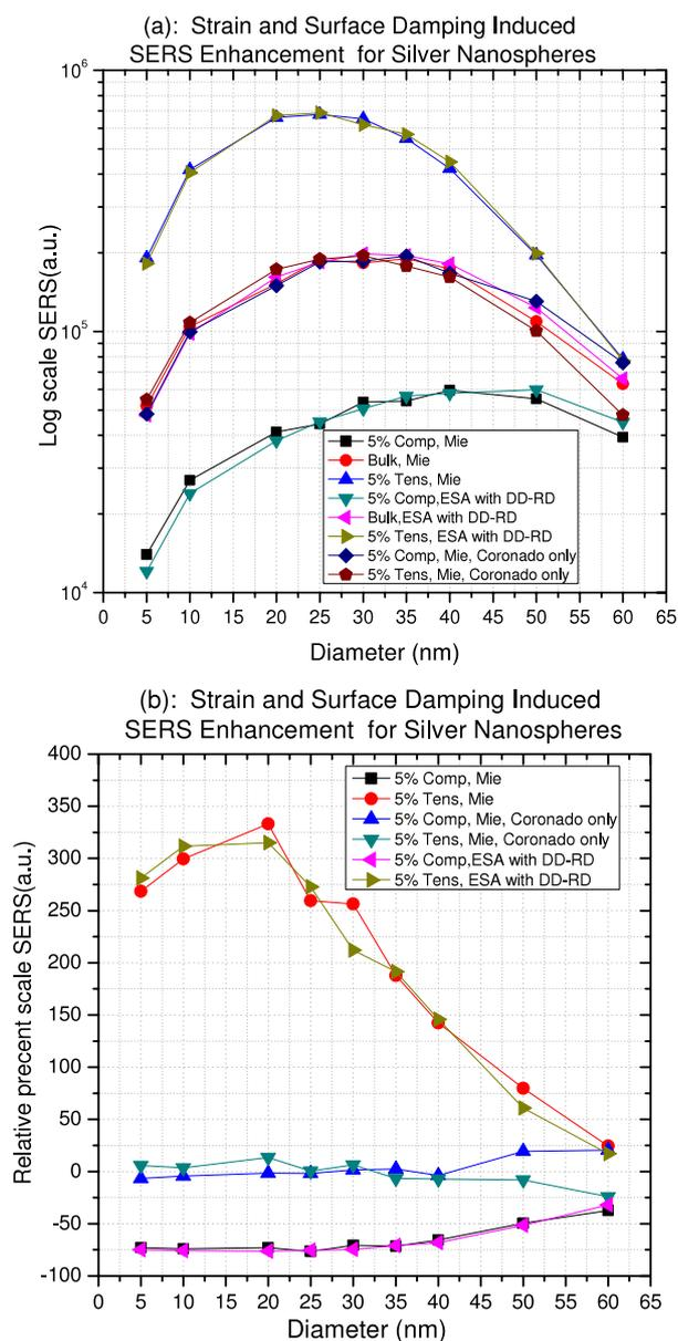
**Figure 3.** Strain effects on SERS enhancements of spherical silver nanoparticles for a range of nanoparticle diameters.
