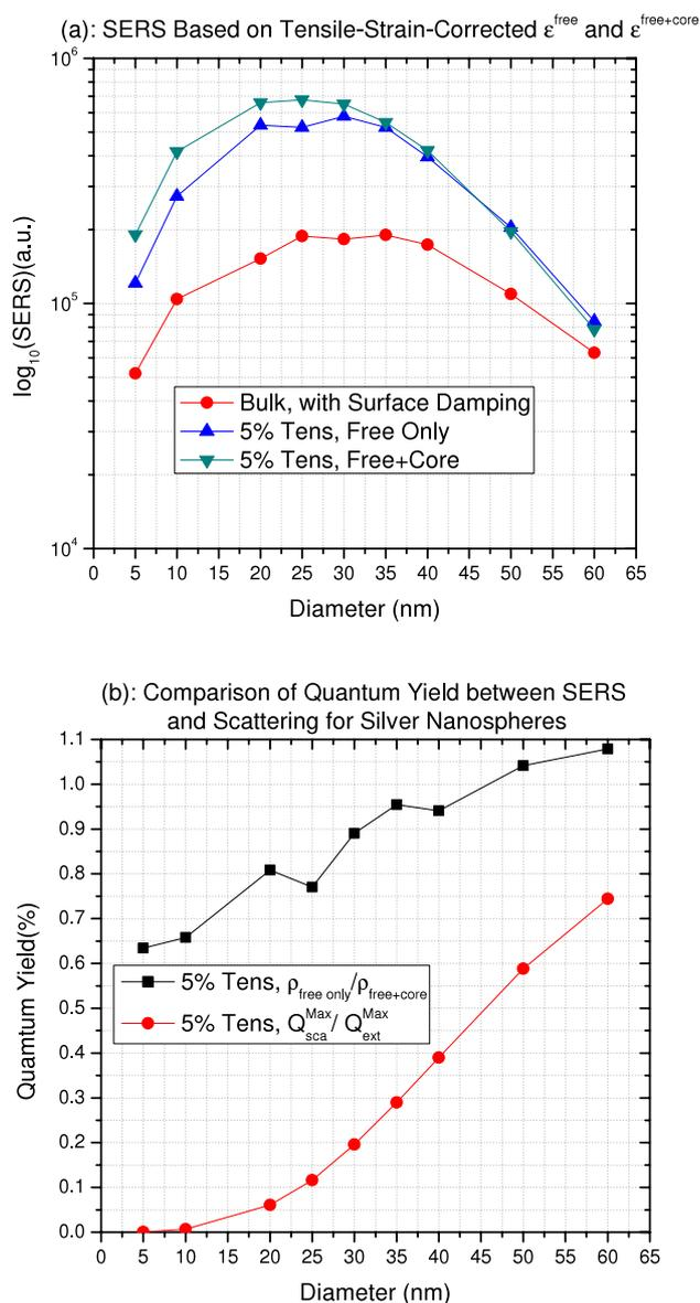
**Figure 4.** (a) Tensile-strain-induced SERS enhancements accounting for free electrons only and both free and core electrons of spherical silver nanoparticles for a range of nanoparticle diameters. (b) Delineation of free electron contribution to the strain-induced enhancement in scattering efficiency and SERS enhancement.
