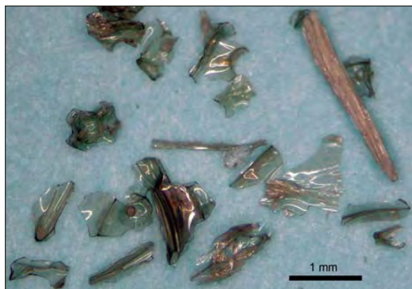
Figure 9. Photograph of glass shards from ALS 00-30. Angular shard morphology is consistent with minimal postdepositional reworking. Evidence for chemical weathering appears minimal: glass surfaces lack evidence for hydration cracking; clay formation is very minor and found only in partially enclosed vesicles on <5\% of examined shards.
