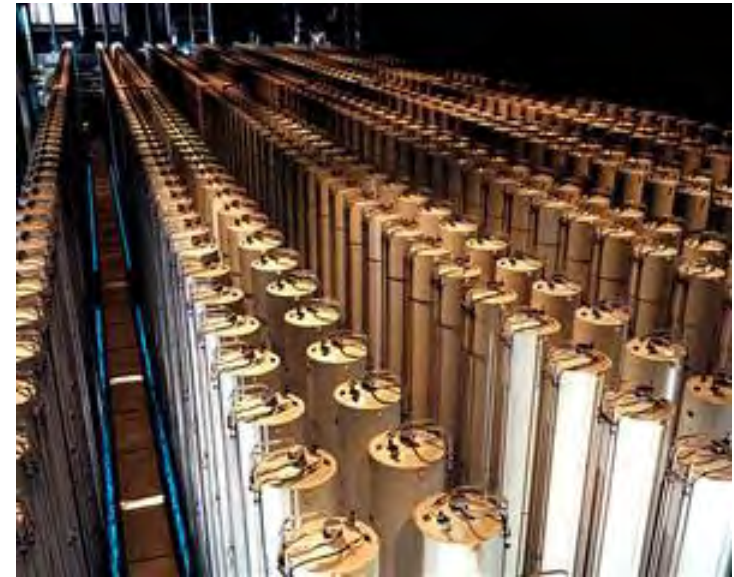
“Aluminum tubes”: centrifuges to separate ^{235}\text{U} from ^{238}\text{U}
