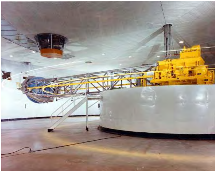
Centrifuge used to train pilots at sustained levels of high gravity (simulated)
