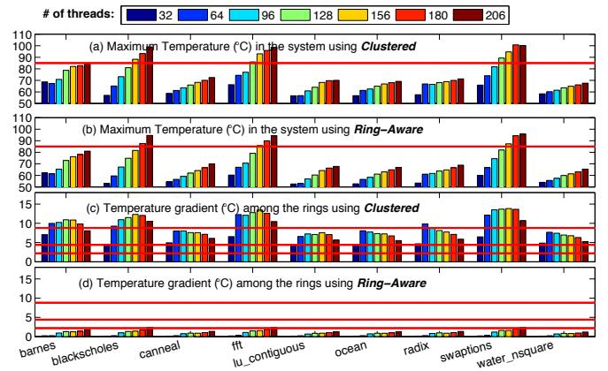
Fig. 6: System maximum temperature and ring temperature gradient using *Clustered* and *Ring-Aware*.
