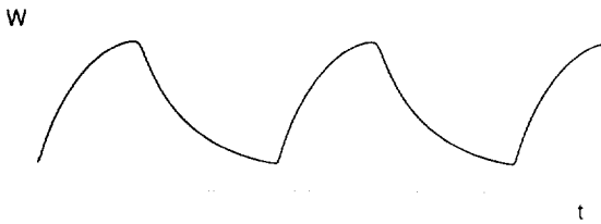
Fig. 5. Slow variable time course for the Morris–Lecar oscillator. The time required to traverse a w interval increases as threshold (a “knee”) is approached. This “scalloped” shape of the time course ( w' \cdot w'' < 0 ) satisfies Hypothesis C.
