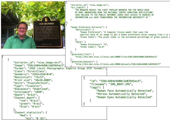
Figure 2. An example of the type of metadata returned by the DTS, in this case given an image file. The DTS returns a breadth of extracted information in JSON such as EXIF metadata associated with the image; computer vision derived data from the image contents such as faces, eyes, and OCR text; as well as more domain specific information available within the instance such as the green index and human preference score used by our Green Infrastructure use case.
