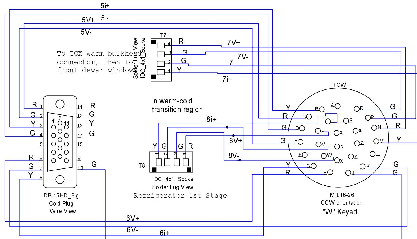
Wires are "quad twisted" twin pairs from LakeShore Cryogenics.
