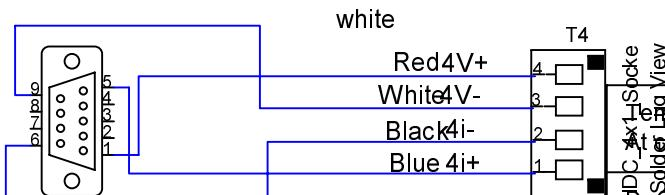
Temperature Sensor Cable MS16-26 normal keyed plugs at each end. Twisted pair cable (8 pairs) connecting plugs.
