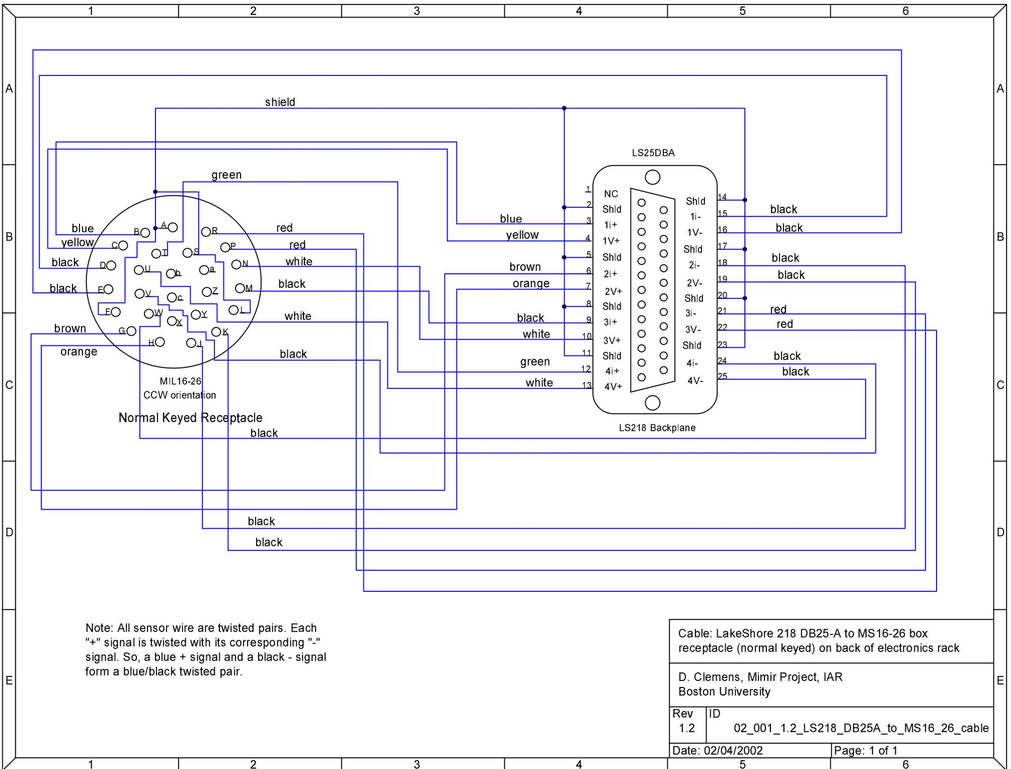
Note: All sensor wire are twisted pairs. Each "+" signal is twisted with its corresponding "-" signal. So, a blue + signal and a black - signal form a blue/black twisted pair.
