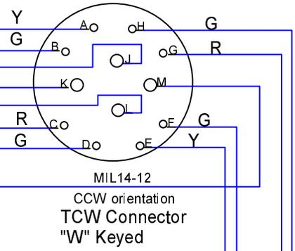
Temperature Controller Warm to Cold Bulkhead Cable ("W" keyed hermetic receptacle) to DB15HD plug
