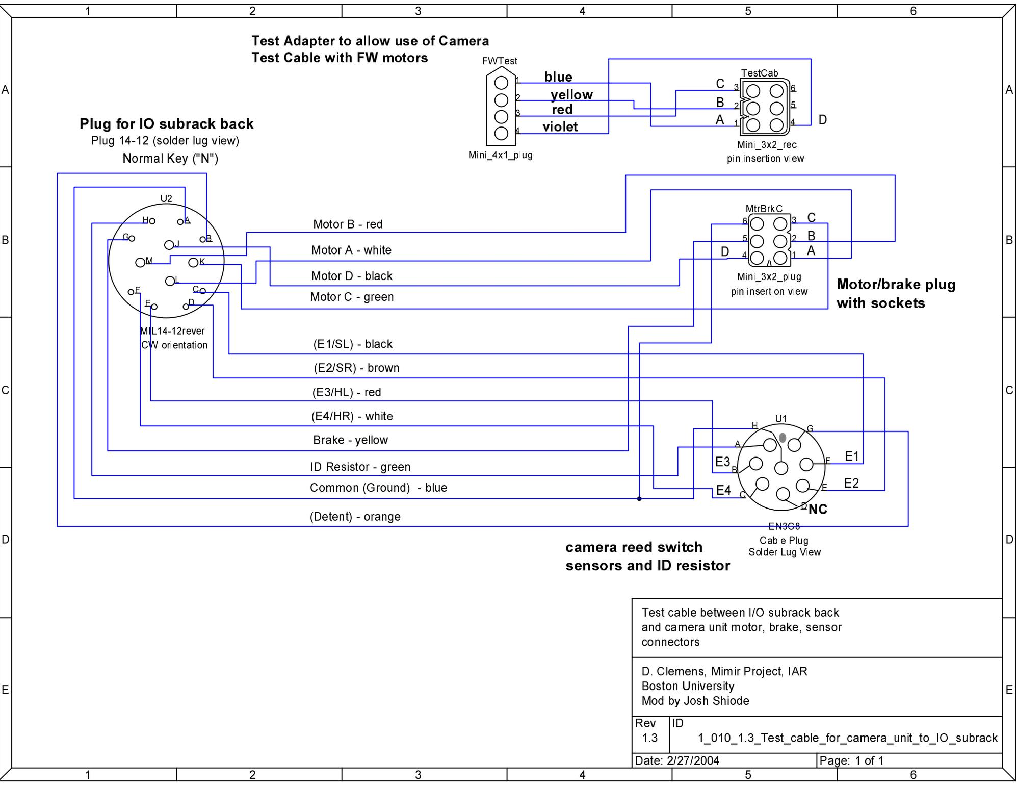
**Test Adapter to allow use of Camera Test Cable with FW motors**
