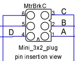
**Motor/brake plug with sockets**
