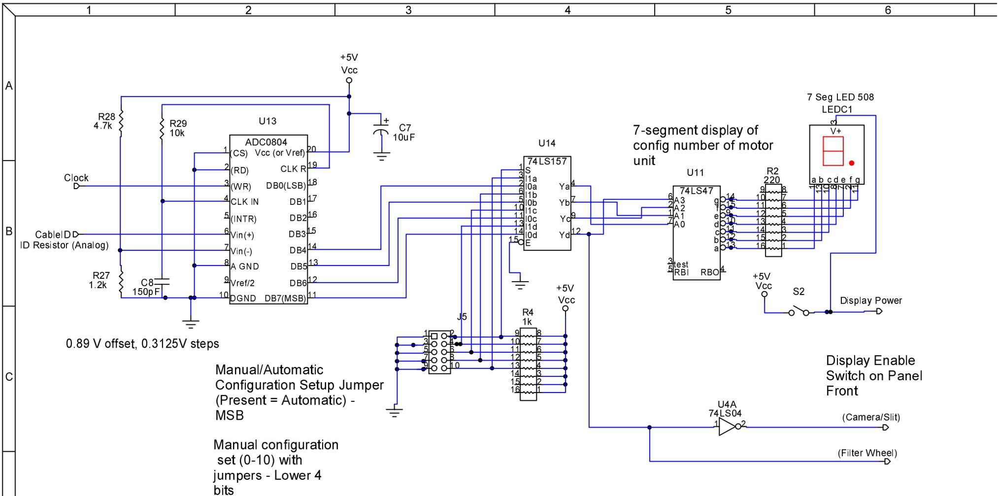
Configuration Decode and Display - Latches new configuration from either the comparitor output or the manual jumpers when the clock line goes low.
