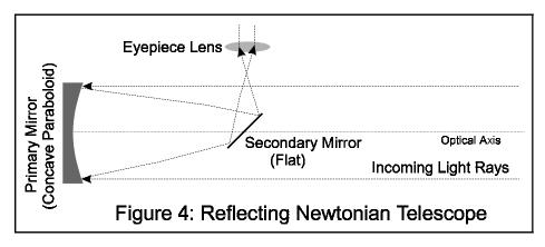
The first telescope design that used mirrors instead of lenses was invented by Isaac Newton 1680. The in objective in this design (see Figure 4) is a concave parabolic mirror, which reflects light onto a flat secondary mirror, moving the focus of the primary outside of the path of the light rays entering the
