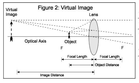
Note: The dashed lines in each figure represent a few of the numerous light rays leaving from a single point on the object. The rays that fall upon the lens are bent to form an image. For simplicity, these diagrams show only three rays from one point at the top of each object.
