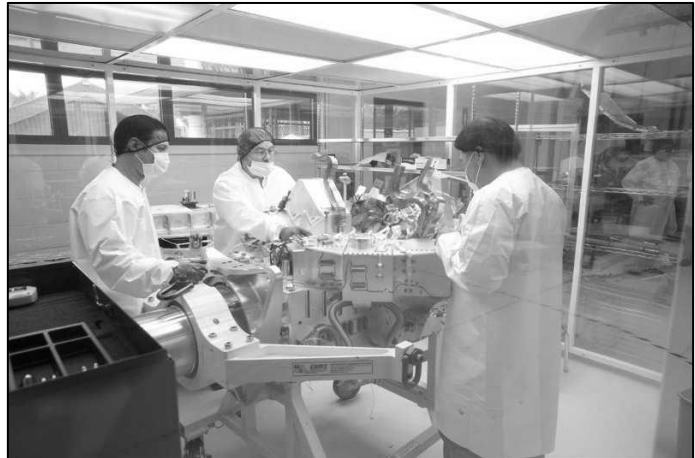
Figure 5. Disassembling and cleaning the GNIRS optical bench.
