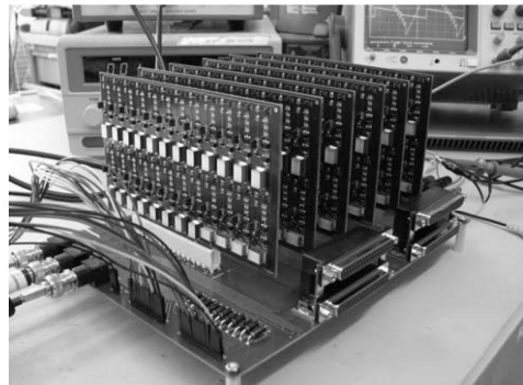
Figure 5. 144-channel prototype of a high-voltage MEMS array driver
