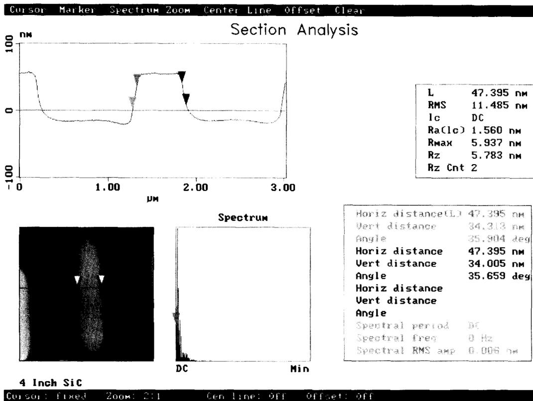
**Figure 8** Atomic force microscope scan of an ion-machined CVD SiC stamper, showing excellent feature definition and smooth side walls sloping at ~35°
