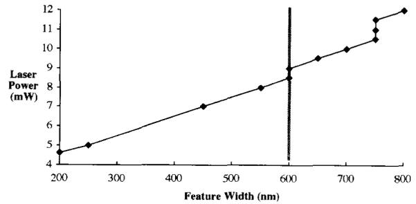
**Figure 4** Feature width in developed photoresist as a function of incident laser power from the laser beam recorder system; results shown are for 680-nm thick JSR NFR-012R negative tone photoresist on CVD SiC; Desired feature width is 600 nm
