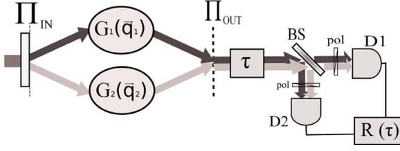
FIG. 1. (Color online) Scheme of the proposed setup. Horizontally polarized photons from type-II SPDC are assigned a phase dependent on the photon transverse momentum  $\phi_o(q_o)$ , while the vertically polarized ones are assigned a phase  $\phi_e(q_e)$ . The modulated photons enter a type-II quantum interferometer, which records the coincidence count rate as a function of the delay  $\tau$  between the photons given by an appropriate delay line.
