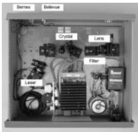
Figure 1: Example of a compact twin-photon source.
