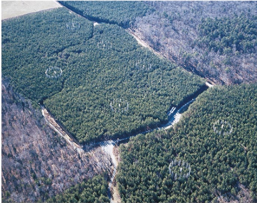
FIG. 3. FACE (free-air CO 2 enrichment) site in loblolly pine forest, Durham, North Carolina. Each experimental plot is 30 m in diameter. Six plots are used in the replicated experiment, while the seventh plot (at upper left) is a prototype used to refine FACE technology. (Photo by Will Owens.)
